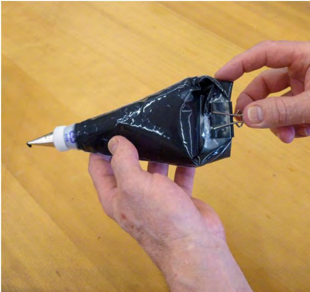
(8) After the end has been folded a few times, then I also fold over the edges and put a large binder clip onto the end to hold it. You can keep the mixture in the bag for a couple of weeks - just put a push pin into the tip to plug the hole. If the goop separates from the glass powder you might be able to massage it in the bag and get it to work, or put it back into the bowl, mix, and the reload or put into a new bag.
