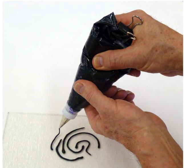
(9) You just barely need to squeeze the bag to get it to flow out. If it is too thin and the line spreads out on the glass, then you need to squeeze the mixture back into the mixing bowl and add more glass powder. If it is too stiff, add more goop. If you line spreads you can also quickly set it with a hair dryer. Clean the tip with water and a metal wire if it plugs up.
