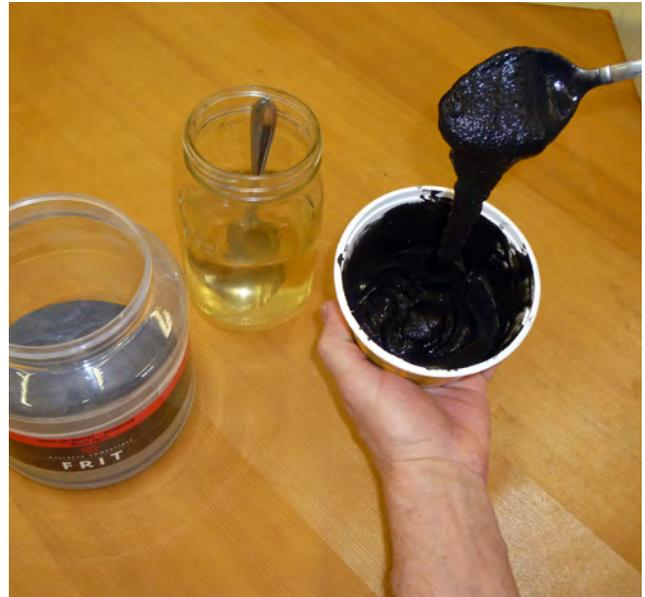
(5) Mix the powdered glass (I use 08 size Bullseye Glass frit) with the goop in a plastic container. I describe how to make the CMC goop on the first page. Wear a dust mask (NIOSH 90) that can handle silica dust.
